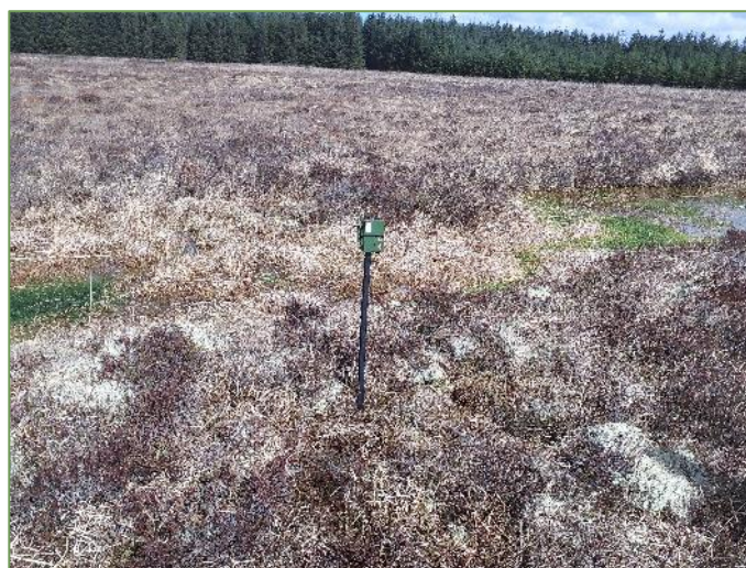
Plate 2.1 - Song Meter Mini Bat Ultrasonic full-spectrum detector deployed at the proposed Turbine 4 location.
